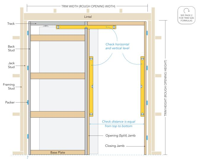
Run straightedge or láser line across front edge to ensure Opening Jamb and Closing Jamb are flush with each other and the wall
